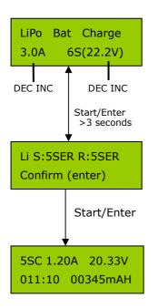
The value on the second line sets a charge current and the voltage of the battery pack.
